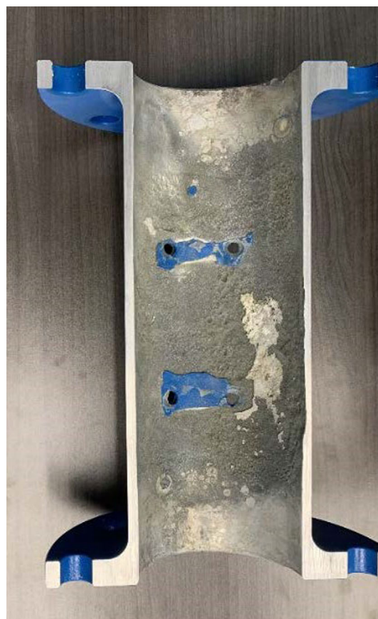
FIGURE 4 Example of pitting in a metallic flow cell when the non-conducting layer has eroded. Photo provided by LiquiTech with permission.
