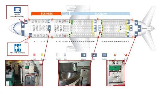
Figure 1. Depiction of the arrangement of water supply points inside an Airbus model aircraft.
