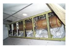
Figure 2. Aircraft potable water tank.
